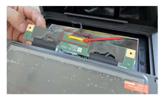
**Step 4**Raise the lever that holds the cable in place
